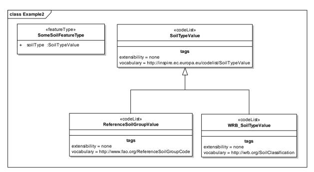
Figure 13 – A non-extensible code list super-class: Only values from the ReferenceSoilGroupValue or from the WRB\_SoilTypeValue code lists may be used for the soilType attribute of SomeSoilFeatureType.
