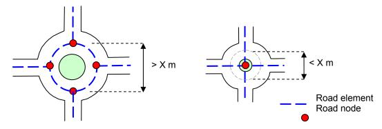
Figure 18 – Example of a roundabout with the limit of 25 meters for the outer diameter, as a level for generalisation.
